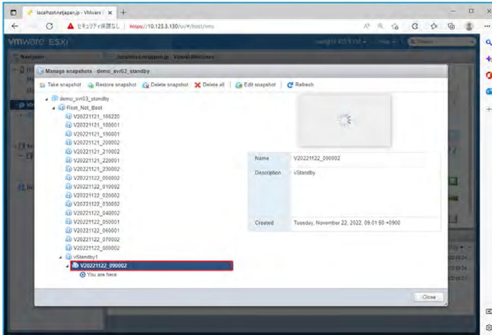
22. Once restoring the latest snapshot completes, boot up the virtual machine and configure the network settings, etc. This is the end of the operating procedures for migrating from the backup of migration source server to VMware vSphere (ESXi) host by using ActiveImage Protector's HyperStandby feature.
