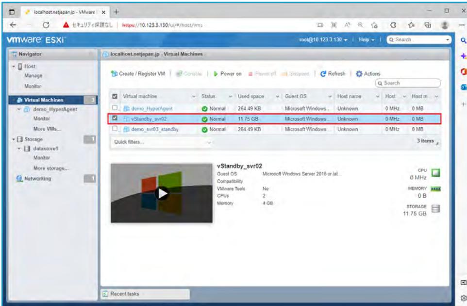
15. In this example, the incremental disk changes of the source machine are taken on a 60-minute interval and added as checkpoints to the virtual standby machine. These snapshots of the virtual standby machine can be restored for migration.
