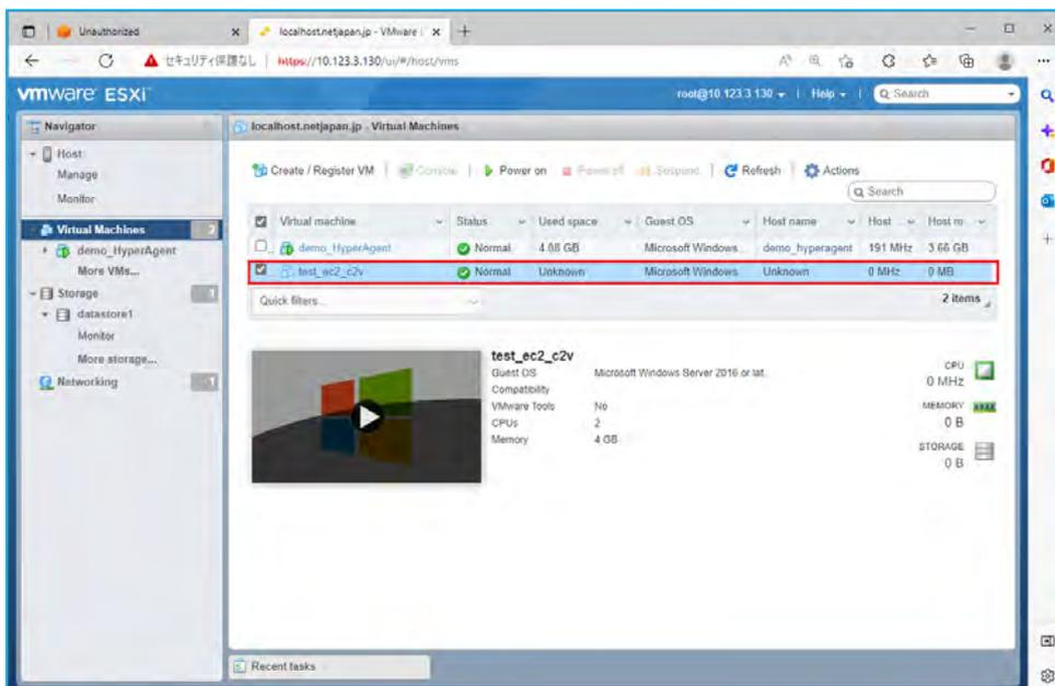
3. Insert the Windows RE-based boot environment media created by using ActiveImage Protector's BE builder to the newly created virtual machine "test\_ec2\_c2v" and boot into the recovery environment. Please wait until recovery environment completely boots up.
