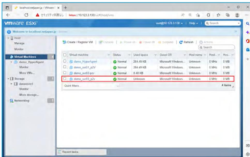
3. Insert the Windows RE-based boot environment media created by using ActiveImage Protector's BE builder to the newly created virtual machine "demo\_svr03\_p2v" and boot into the recovery environment. Please wait until recovery environment completely boots up.
