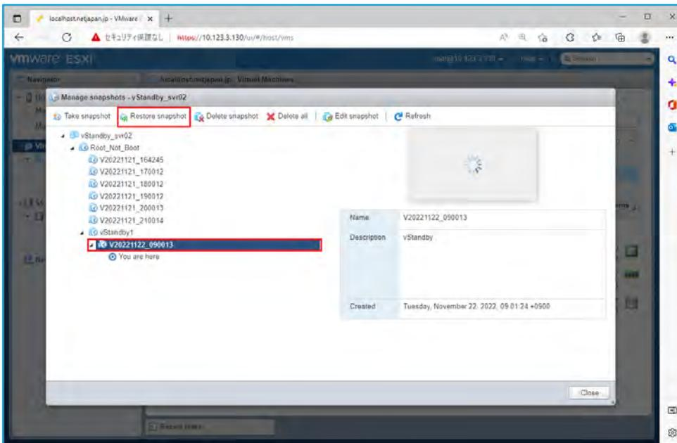
16. Once restoring the latest snapshot completes, boot up the virtual machine. This is the end of the operating procedures for migrating from the source server disk to VMware vSphere (ESXi) host by using ActiveImage Protector's vStandby feature.
