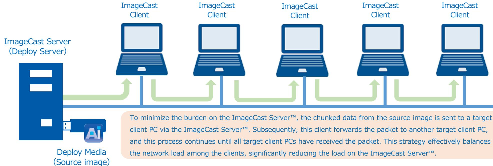
Using stand-alone deployment tool equivalent to the predecessor product ActiveImage Deploy USB, a single click quickly deploys the source image to target computers, eliminating the need for network connection and distribution server. You only need to plug in the created Deploy USB media, power-on the computer and you can deploy the embedded source image of the preconfigured computer system to new client PCs. You can deploy a source image to a small number of PCs even in a meeting room.
